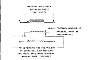
fig. 9. Circuit for measuring balun inductance and calculating the coefficient of coupling between main and tertiary windings.
