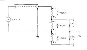
fig. 4. A 3-winding transmission line balun drawn as an auto-transformer. Though shown as an autotransformer it is still a transmission line device. The input versus load impedance relationship follows the transmission line equation and not the transformer law.
