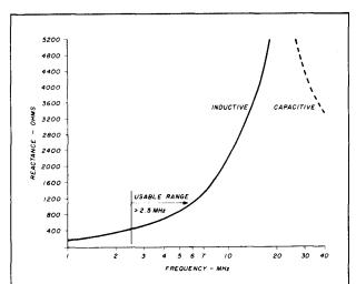
fig. 8. A typical balun reactance versus frequency characteristic. Isolation is at least five times the characteristic impedance from 2.5 MHz to above 40 MHz.
