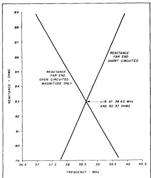
fig. 7. Open/short circuit curves of a balun transmission line showing a characteristic impedance of 82.97 ohms and a l/8 length at 38.63 MHz.
