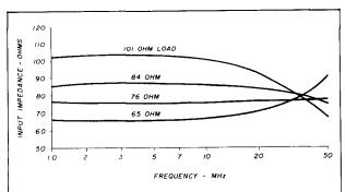
fig. 6. Input impedance versus frequency for 65, 76, 84, and 101 ohm load resistors.
